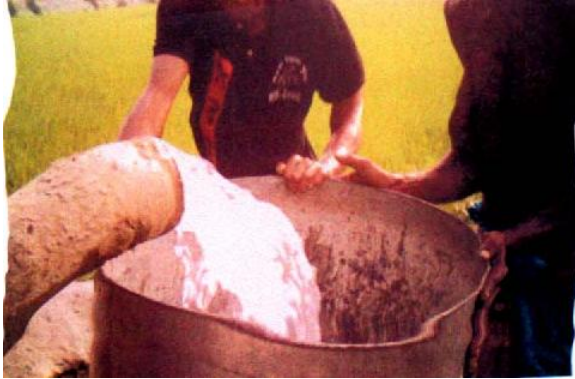
Figure 2: Pump discharge measurement of STW
