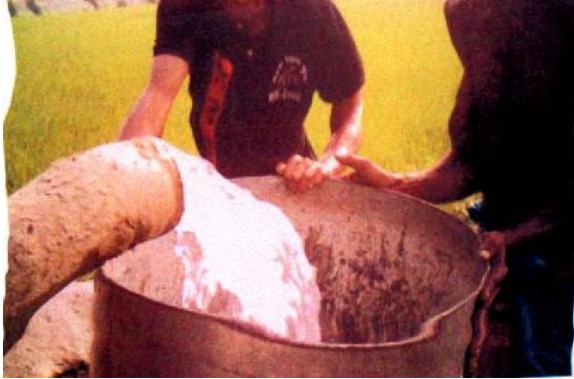
Figure 2: Pump discharge measurement of STW
