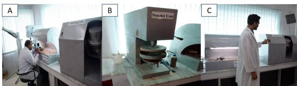
**Figure 1:** Nuclei making equipment A. Shell cutting unit B. Nuclei unit C. Polishing unit
