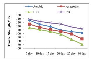
Figure 8: Effect on Fiber strength of banana pseudo stems fiber for different treatments
