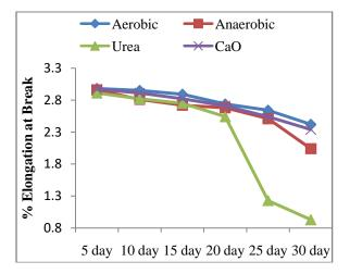
**Figure 10:** Effect on elongation break of banana pseudo stem fiber for different treatment
